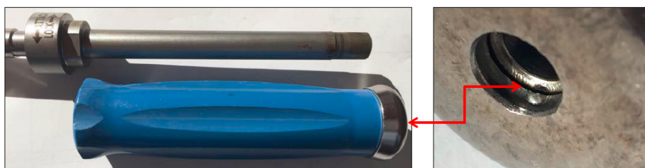
Figure 1: Rupture de la soudure laser
