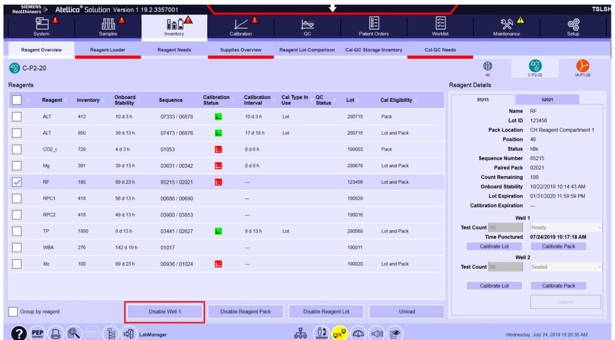
The screenshot displays the 'Reagents' overview table and the 'Reagent Details' panel for the RF reagent. The 'Disable Well 1' button is highlighted with a red box.
