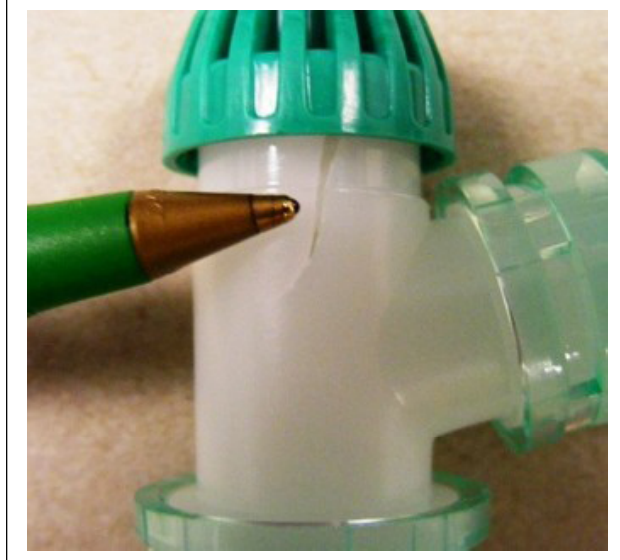
Photo of the crack.
