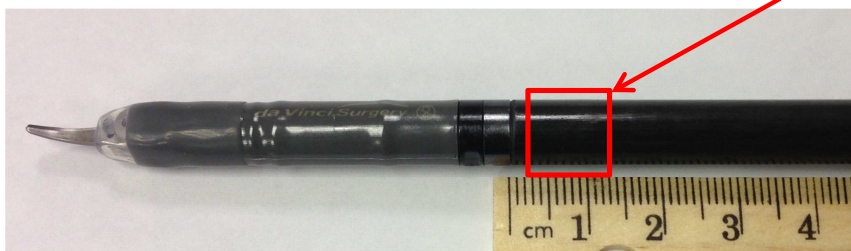
Figure 1: Localisation des micro-fissures
