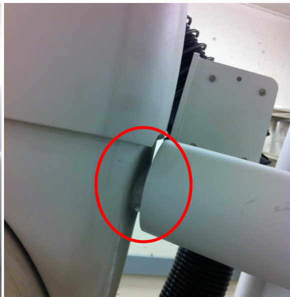
Figure 4 Espace trop large
