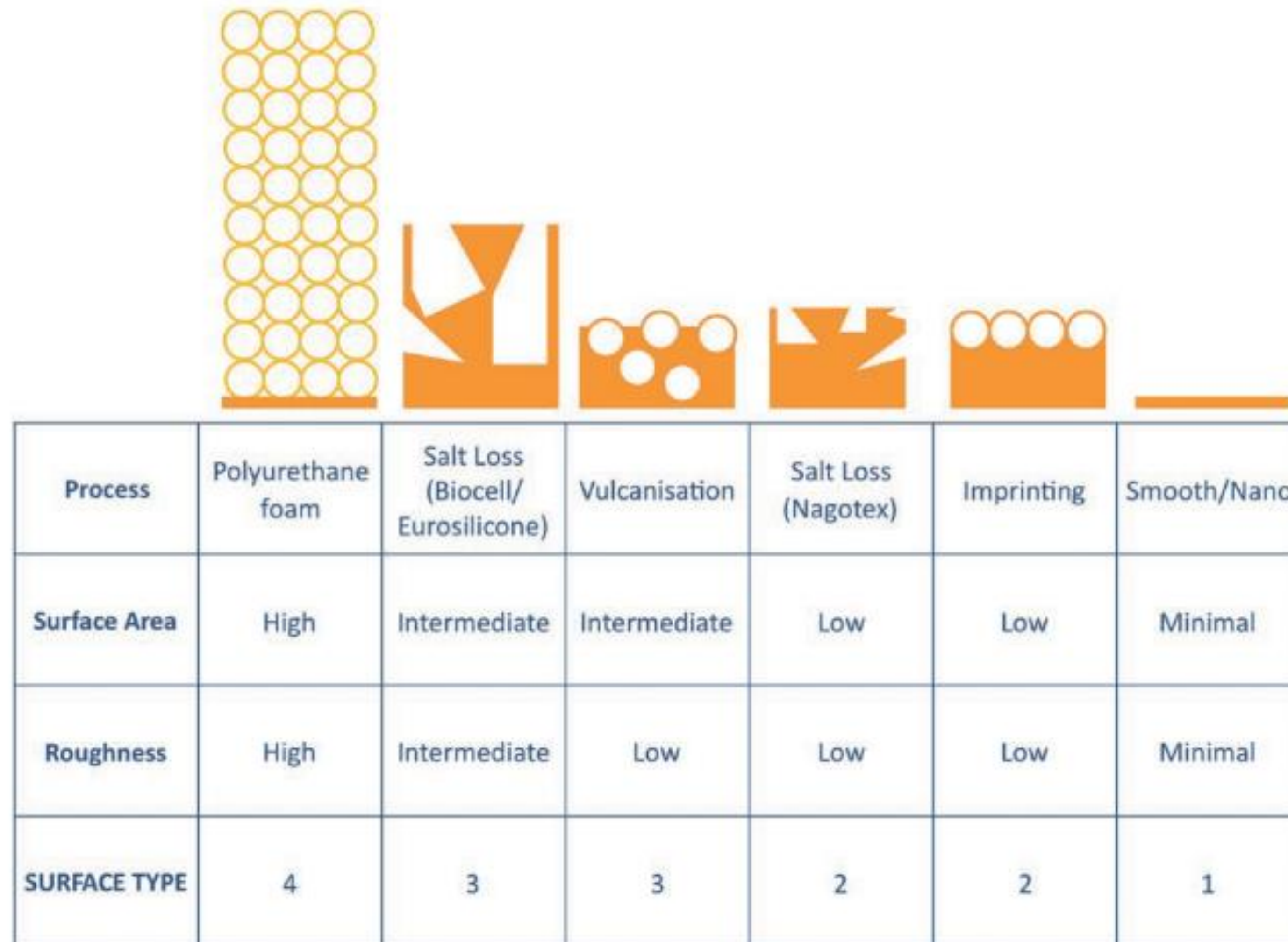
Fig. 8. Implant surface classification relating manufacturing method, surface area, and surface roughness.
